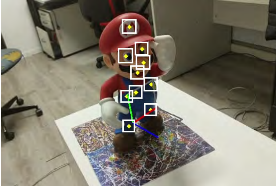
Figure 2.18: The white squares around each yellow keypoint are patches. Notice that here the patches are all very similar in dimension since the distance to the camera for all of them is approximately the same.
