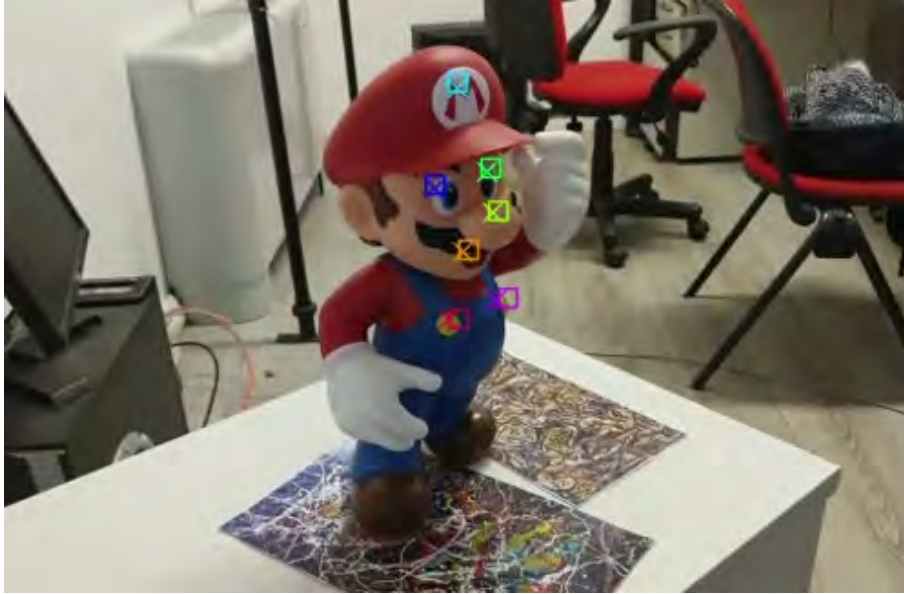
Figure 3.5: Here the colored squares are the projected groundtruth, the colored crosses are Yolo detection’s centroids, used afterwards to calculate PnP. The
