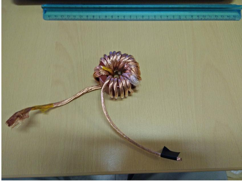
Figure 4.2: Example of final toroidal inductor
